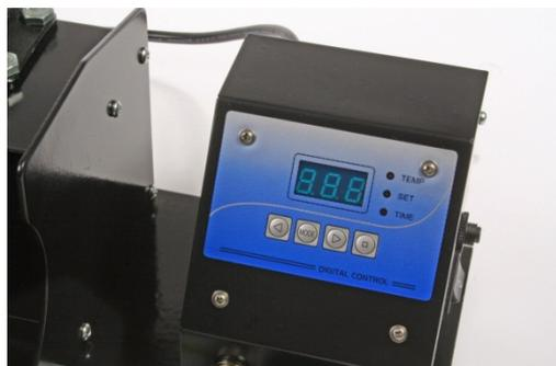
3) As per the supplied instructions adjust the press for the circumference of your mugs. Turn on the mug press and set to 180°C idle temperature and a pressing temperature of 185°C. The pressing time should be 15 seconds.
