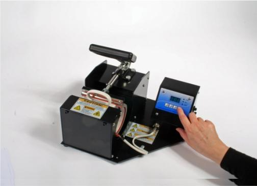
6) Insert the mug in the press close the handle and press the square start button. The temperature will fall before rising to the press temperature of 185°C and the time will only then count down.
