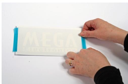
4) Place the image face down and add heat tape to either side
